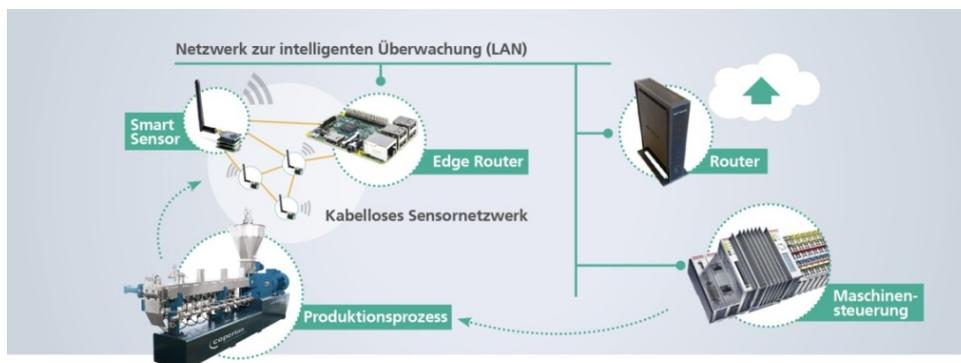
Scientists at the Fraunhofer LBF have developed an intelligent sensor node-based monitoring and optimization system for production lines using twin-screw extruders. This opens chances for predicted maintenance in production processes and thus reduces stand still times.
